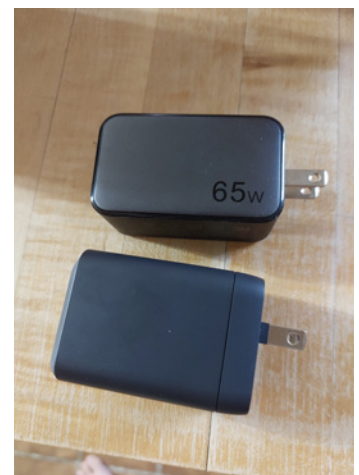
GaN chargers promise more energy efficiency than existing silicon-based chargers (Clayton Ou)
