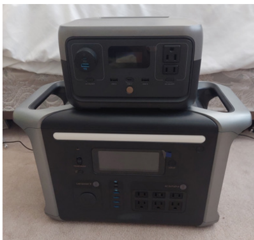
Portable LiFePO4 power stations that can be charged with (separate) solar panels (Clayton Ou)
